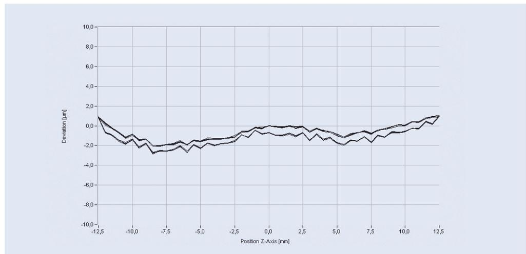
The positioning accuracy of a precision H-824 Hexapod in Z direction over the complete travel range of 25 mm is a few micrometers, and the repeatability is considerably below  $\pm 0.1 \mu\text{m}$
