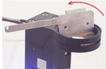
Figure 4: Tightening the objective insert with the wide face of the flat wrench
