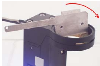
Figure 5: Unscrewing the objective insert using the wide face of the flat wrench
