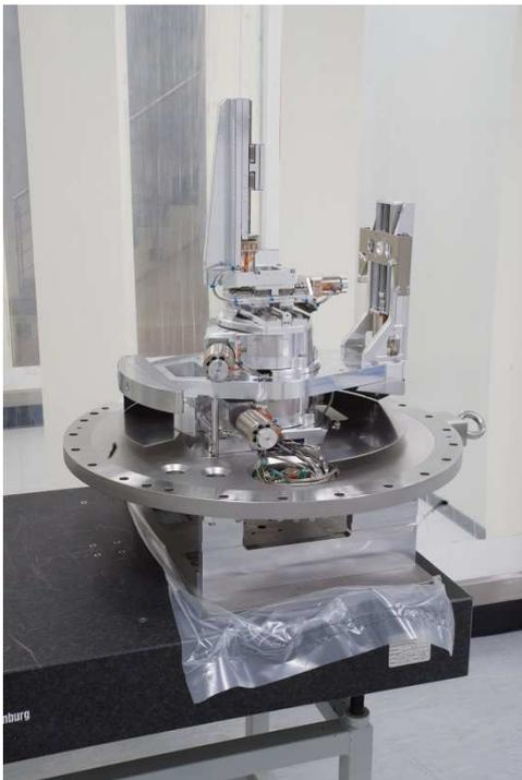
Fig. 1 Multi-axis positioning for spectroscopy, manufactured in a cleanroom in Eschbach according to the ISO 7 classification
