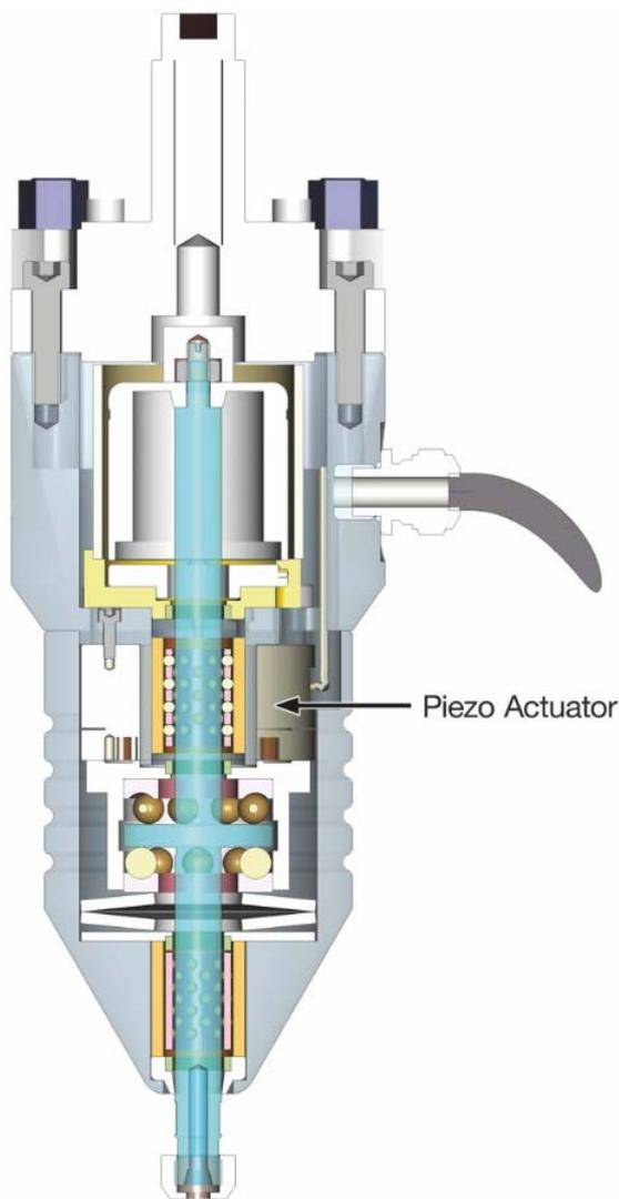
Fig. 7 The piezo actuator could be integrated into the vibratory spindle in a space-saving arrangement (Figure: ICT-IMM)
