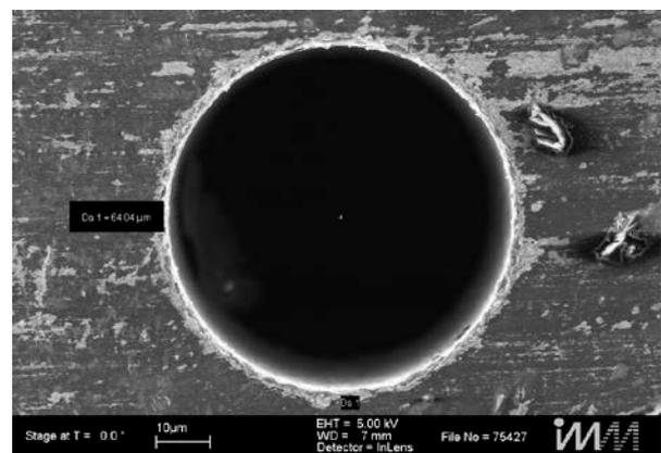
Fig. 2 A hole 64 µm in diameter produced with a die-sinking EDM machine equipped with a vibratory drilling spindle. The deviation from concentricity and cylindricity of the hole is in each case only 1 µm (Figure: ICT-IMM)
