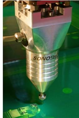
Fig. 1 Sonodrive 300 vibratory spindle (Figure: ICT-IMM)
