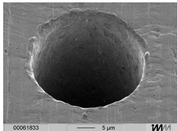
Fig. 3 A hole only 20 µm in diameter produced with a die-sinking EDM machine equipped with a vibratory drilling spindle (Figure: ICT-IMM)
