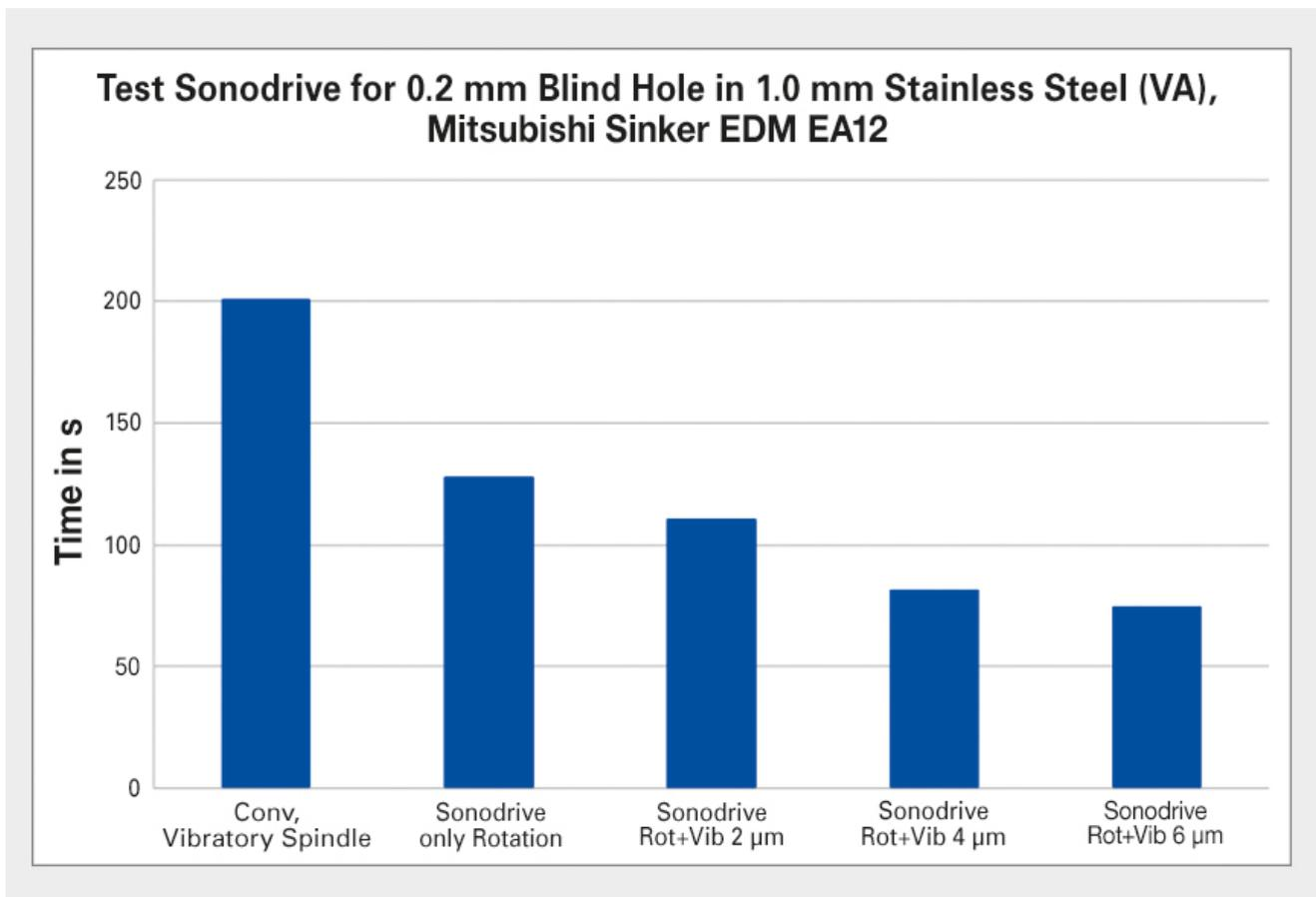
Fig. 4 With a 0.2 mm diameter blind hole in a 1.0 mm thick VA material, the machining time in a test on a EA12 die-sinking EDM machine from Mitsubishi Electric was reduced from 200 to slightly below 80 seconds (Figure: ICT-IMM)
