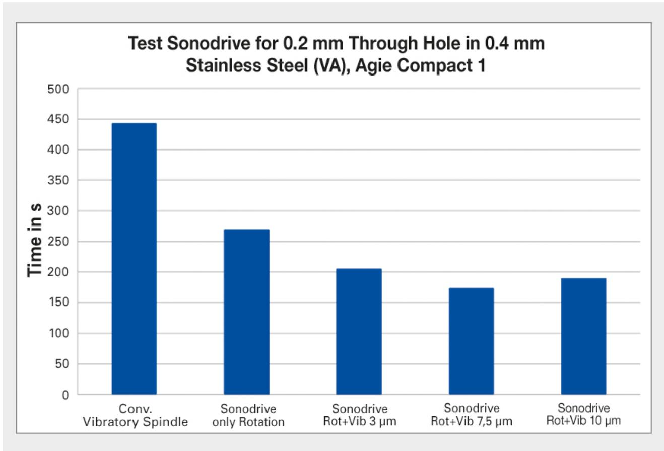
Fig. 5 On an Agie Compact die-sinking EDM machine, the 0.2 mm diameter through-hole in a 0.4 mm thick VA material was also obtained approx. 60 % faster through the use of a vibratory spindle (Figure: ICT-IMM)
