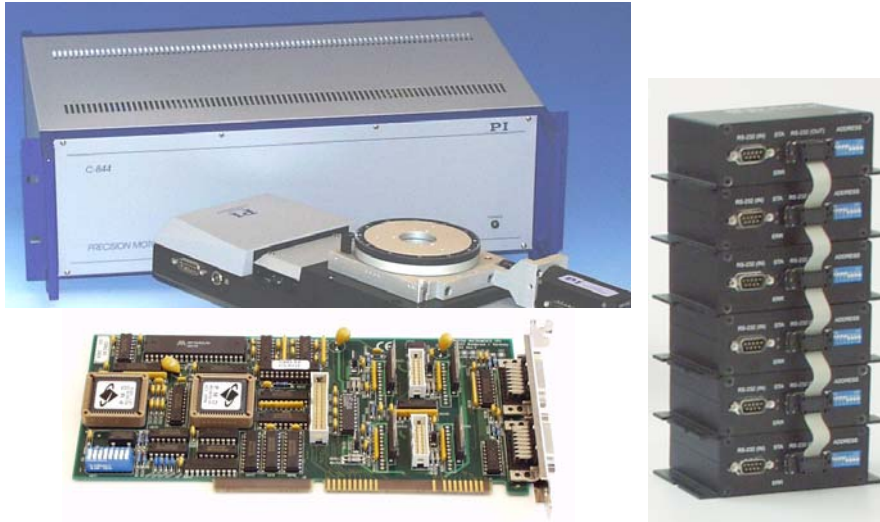
Fig. 21 Discontinued DC-motor controllers: C-844, C-842 ISA bus card and C-862 (black) Mercury®
