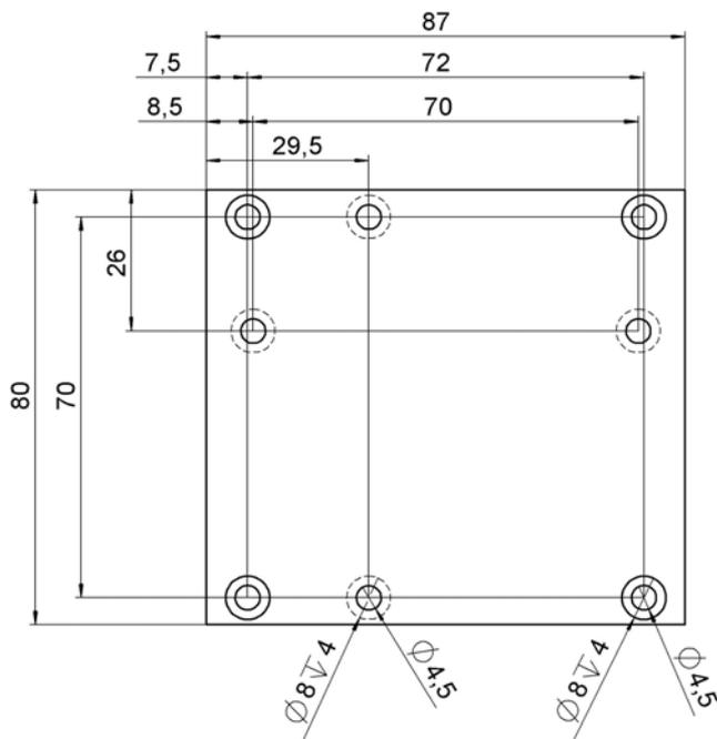
Figure 8: M-403.AP2 Z-axis adapter plate
