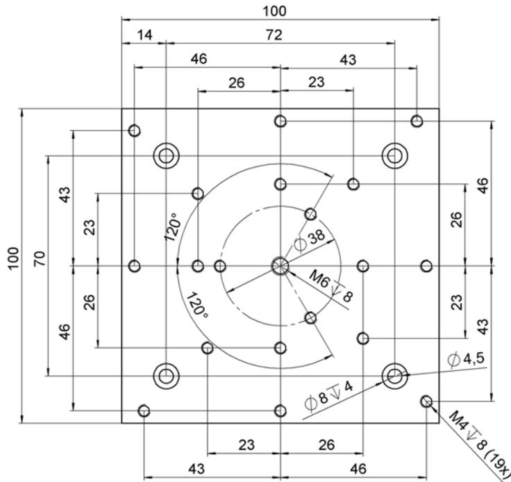
Figure 7: M-403.AP1 adapter plate with PI standard hole pattern
