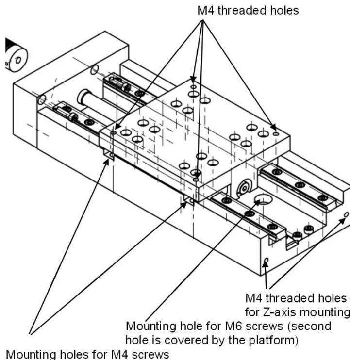
Figure 3: M-ounting hole locations on stage, identical for all models
