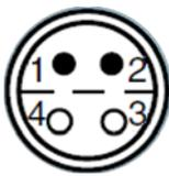
Figure 18: Sensor connection: LEMO connector FFA.05.304.CLAC32Y, contact side
