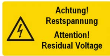
Figure 3: U-624: "Residual voltage" warning sign on connector
